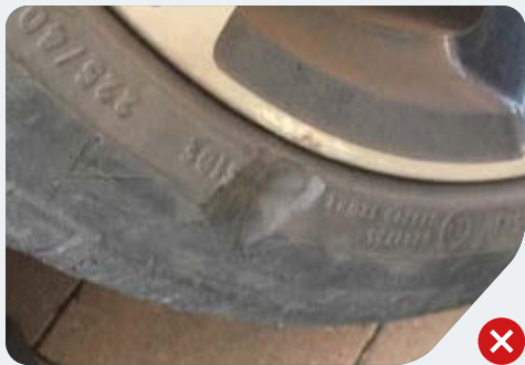
Tyre sidewall damage is not acceptable.
