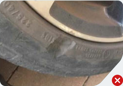
Tyre sidewall damage is not acceptable.
